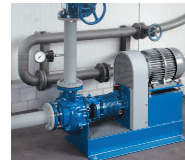
Pump installation with belt drive for viscous media such as oils, paints and adhesives.
